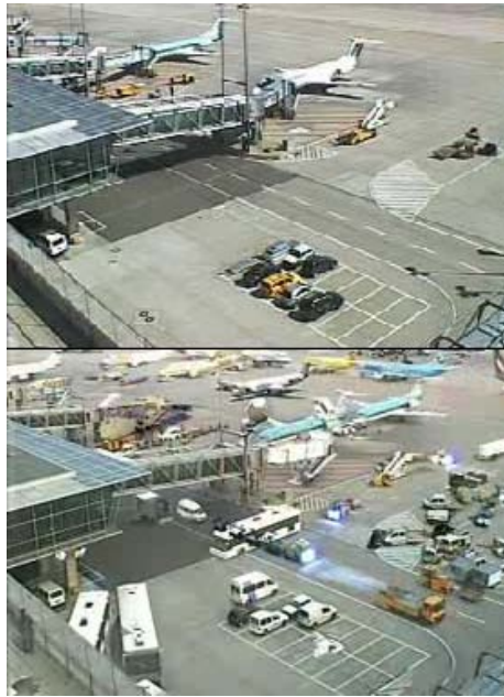
Pictured: Airport gate before Video Synopsis (above) and after (below). 24 hours of footage was compressed into 1 minute of runtime.
